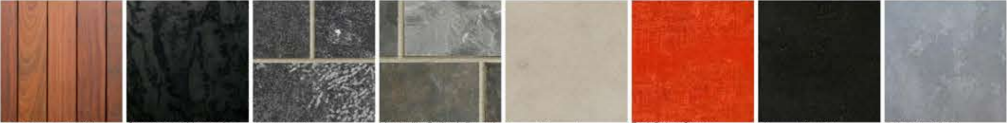
Black Ironwood (Ipé) Cor-ten steel blue patina Marshall's Killkenny Limestone, Flamed. Marshall's Gyrhyd, flamed Precast Concrete Red Ochre Stucco Charcoal Black Stucco Galvanized Steel
