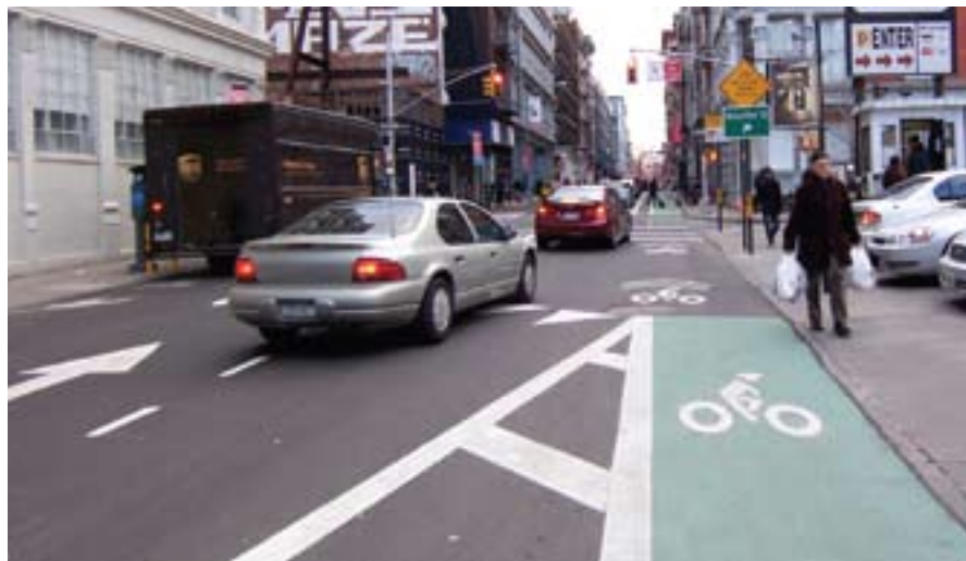
Parking-separated bike path showing mixing zone at intersection: Grand Street, Manhattan
