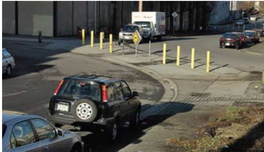
Diagonal diverter: Vancouver, Canada (Credit: Richard Drdul) (Note: for illustrative purposes only)
