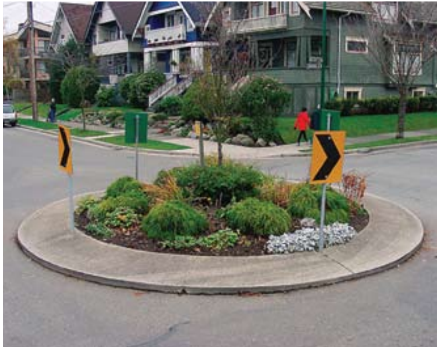
Neighborhood traffic circle with landscaping: Vancouver, Canada (Credit: Richard Drdul) (Note: for illustrative purposes only)
