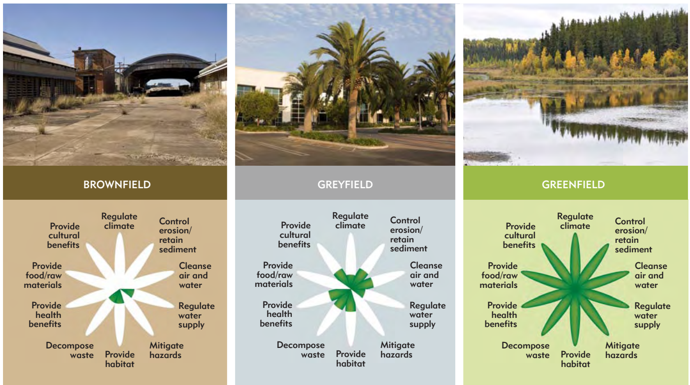
FIG. 2-4. RESTORING ECOSYSTEM SERVICES. A schematic flower suggests how well different types of sites provide ecosystem services, as indicated by the amount of dark green along each petal. In an abandoned and likely contaminated brownfield site ( below left ), ecosystem services are virtually nonexistent, except for what is provided by the scrubby grass and marginal soils. Adding vegetation and healthy soil to a developed, or greyfield, site that would otherwise be dominated by impervious cover, as in a business office parking lot ( below center ), restores nearly all ecosystem services to some degree. The goal of Sustainable Sites is to rehabilitate all sites—including brownfields—so they approach the levels of ecosystem services provided by a natural ecosystem, or greenfield ( below right ).
