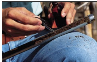
Soil Samples can be collected using a soil probe.
