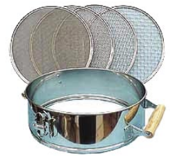
Sieves are one tool used for lab analysis of soil texture.
